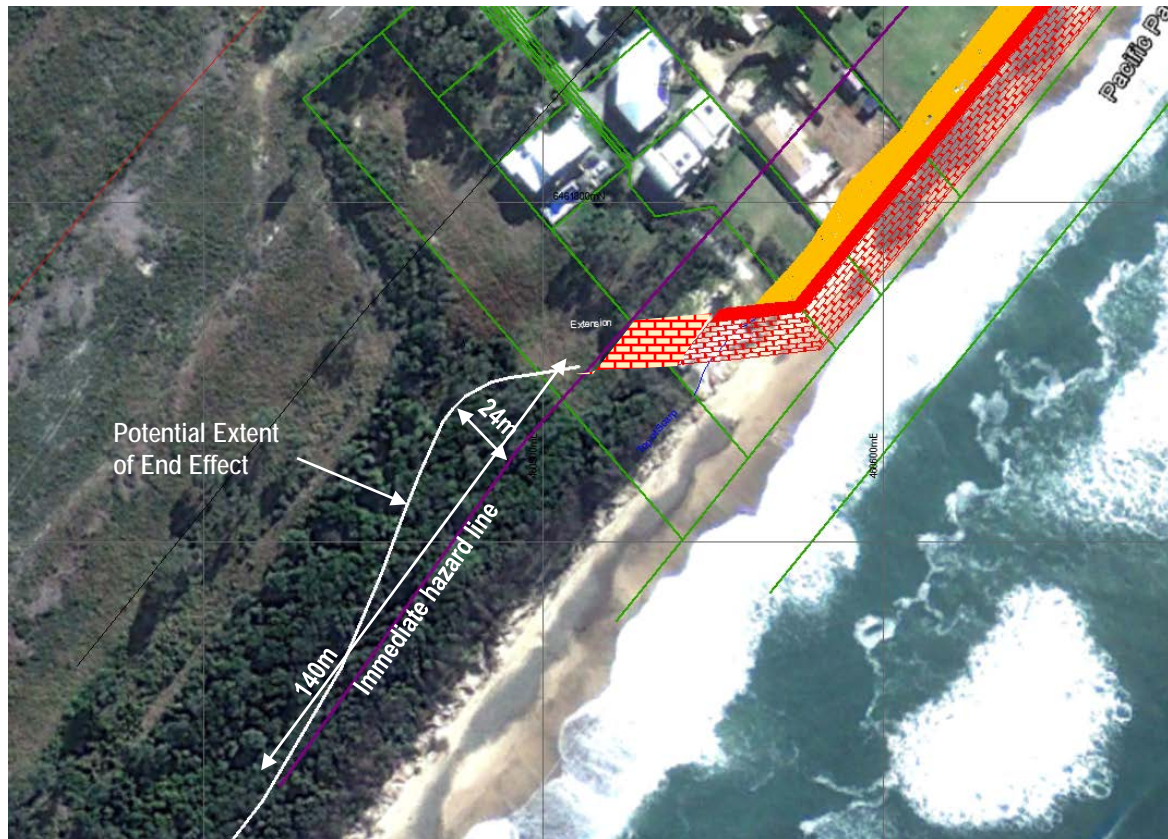
Figure 1 - Area of potential end effects [assuming extension of the wall along preferred alignment]
